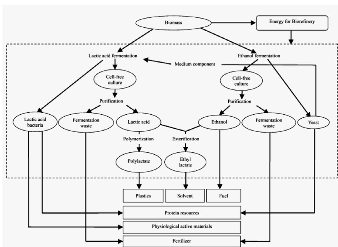
**Figure 1 The biorefinery ecosystem, based on lactic acid fermentation and ethanol fermentation (Ohara, 2003)**
