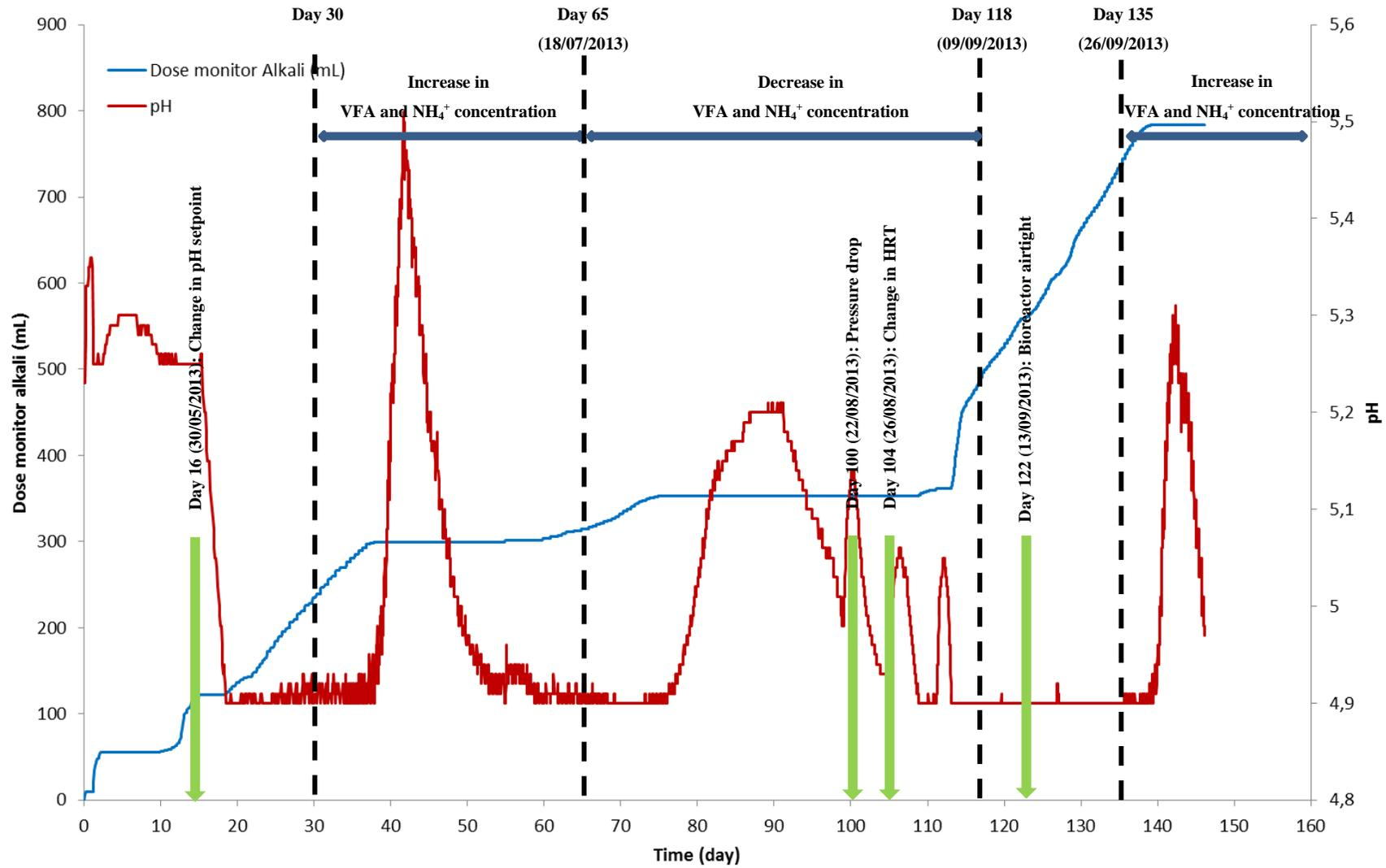
Figure 15 The amount of added alkali (blue line) and pH change (red line) as a function of time.
