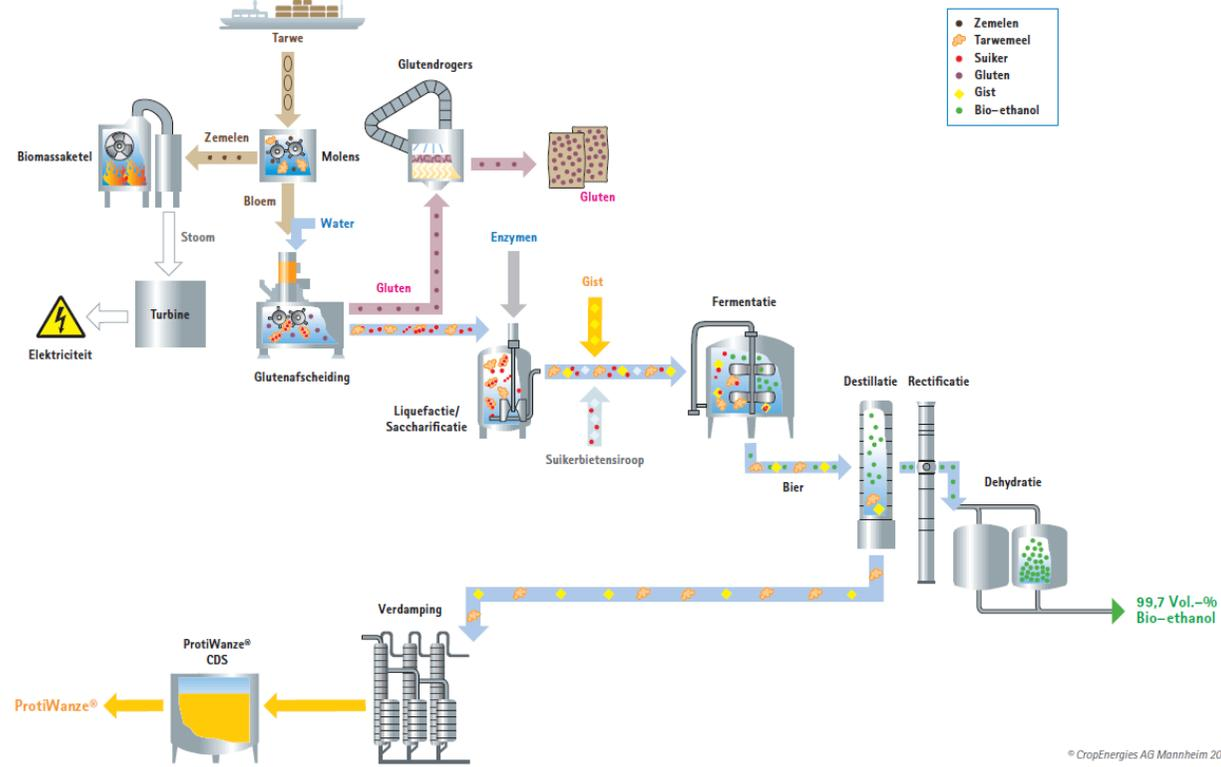
Figure 4 Schematic representation of process scheme at BioWanze, Belgium ([www.biowanze.be](http://www.biowanze.be)).
