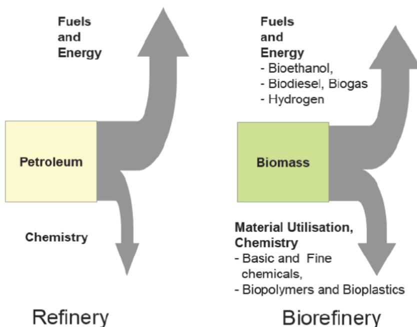
**Figure 2 Oil refinery versus biorefinery (Kamm et al., 2006)**
