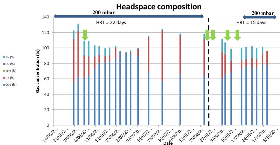
**Figure 16 Fraction of gases as a function of time. Green arrow indicate bioreactor headspace pressure adjustment.**
