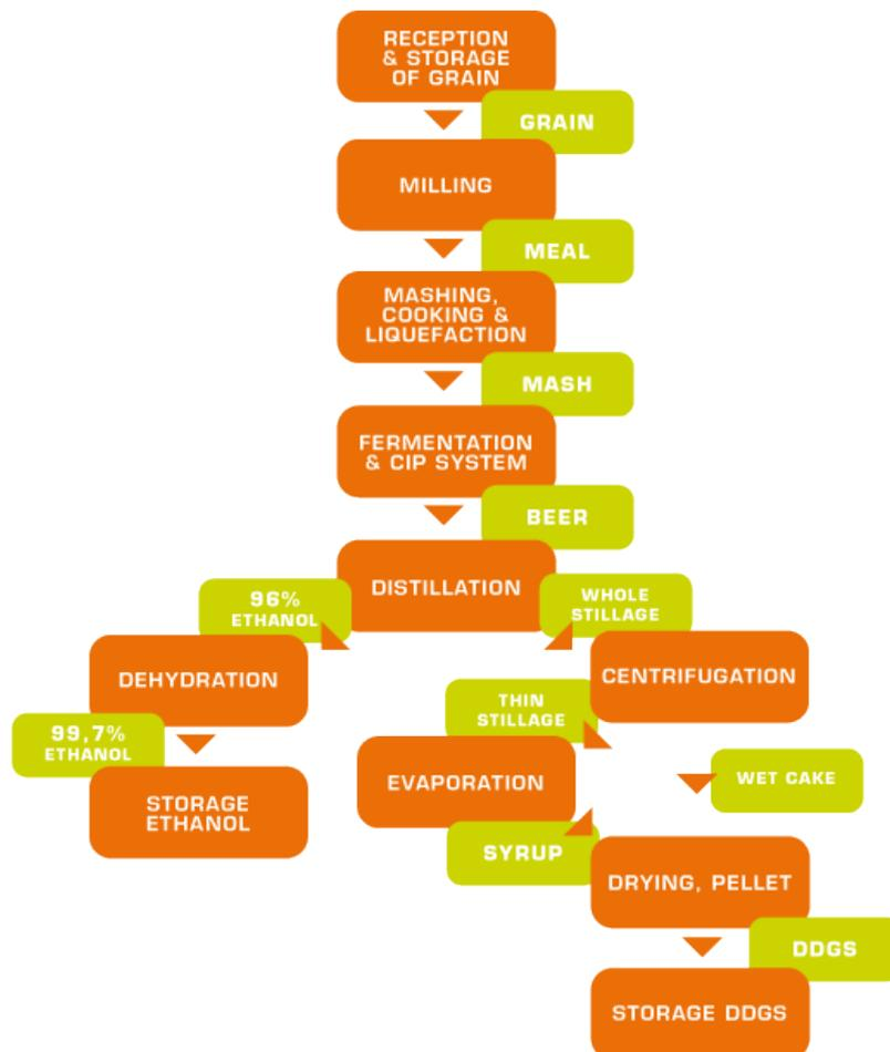
**Figure 3 Production and waste(water) treatment concept at Alco Bio Fuel, Belgium (www.alcobiofuel.com).**
